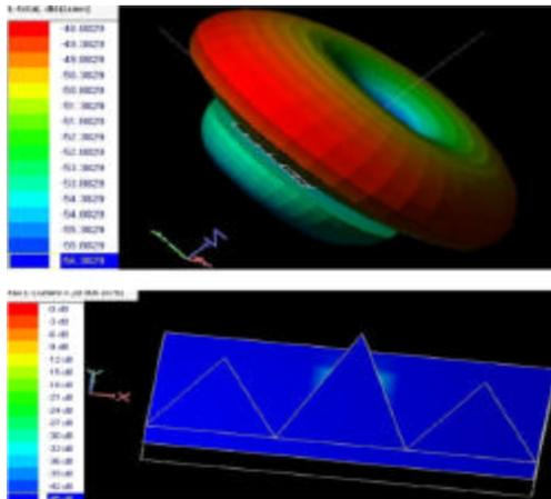
Fig. 6. Radiation pattern & current distribution.
