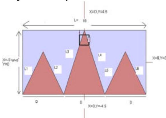
Fig. 7. Triangular shape microstrip antenna.
