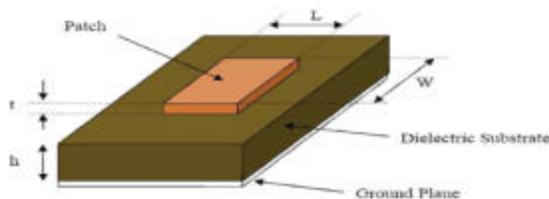
Figure 2.1 Structure of a Microstrip Patch Antenna
